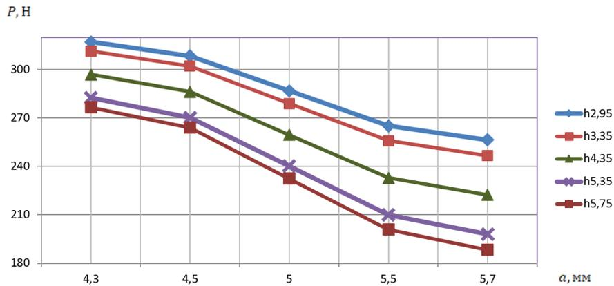
Figure 1: Graph of dependence of total costs  $P$  during felt cutting with the grooved knife with one-sided cross-section on the distance value  $h$ , between transport rollers: while  $a = const$ , in the range  $a_{min} = 4,3 - a_{max} = 5,7$
