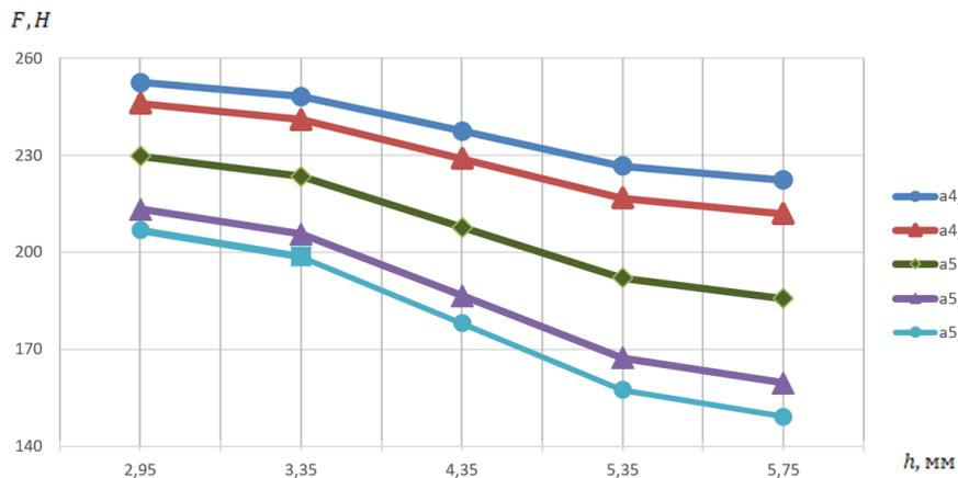
Figure 4: Dependency graph of total costs F during slitting cutting with the grooved knife with one-sided cross-section on the gap size a from the vertical axis of transport rollers to the knife edge: while  $h = const$ , in the range  $h_{min} = 2,95 - h_{max} = 5,75$
