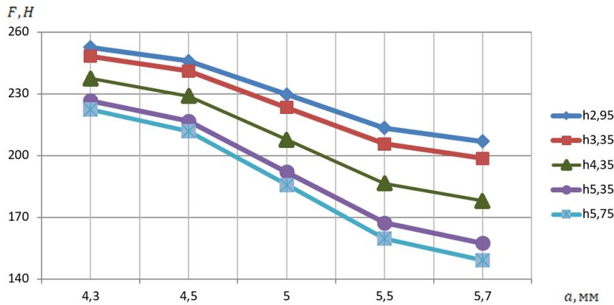
Figure 3: Dependency graph of total costs F during cutting the felt with the grooved knife with one-sided cross-section on the gap size  $h = const$ , between transport rollers: while  $a = const$ , in the range  $a_{min} = 4,3 - a_{max} = 5,7$ .
