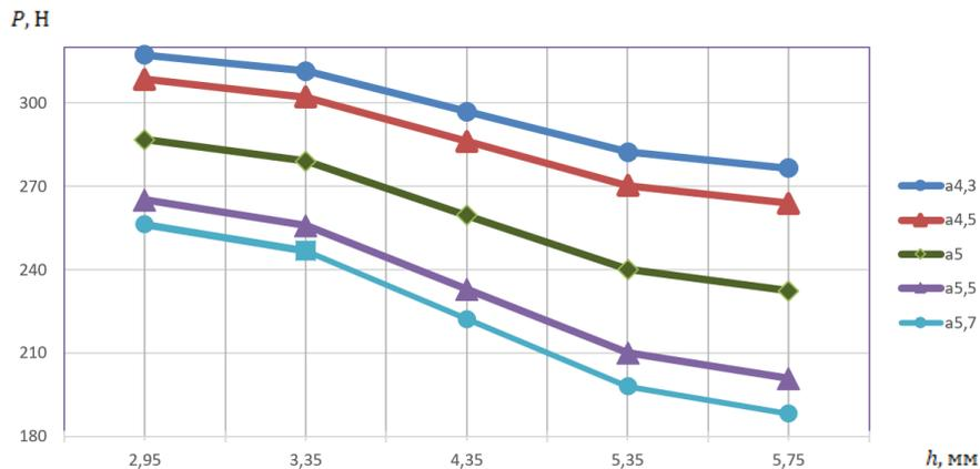
Figure 2: Graph of dependence of total costs  $P$  during cutting of felt with the grooved knife with one-sided cross-section, on the distance  $a$  from vertical axis of transport rollers to the knife edge: while  $h = const$ , in the range  $h_{min} = 2,95 - h_{max} = 5,75$
