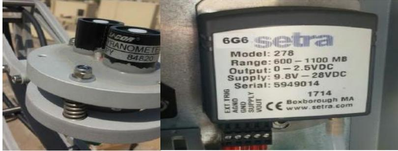
Fig. 4: Pyranometer Unit on RSI Fig. 5: Setra 278 pressure sensor [22]
