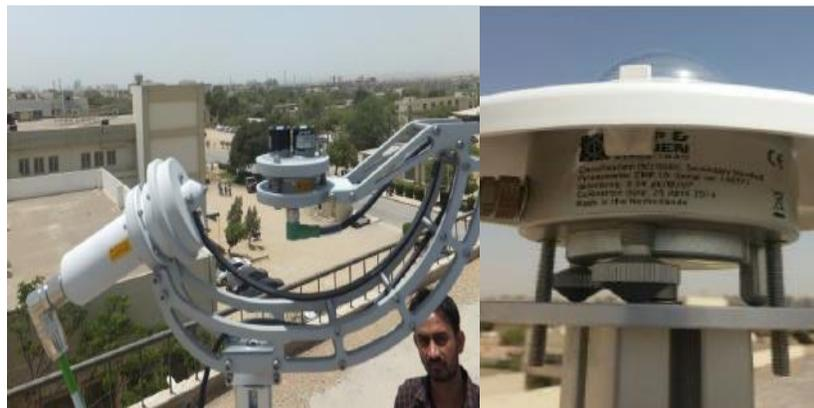
Fig. 2: RSI (red: protection caps) Fig. 3: CMP10 w. sun shield [22]
