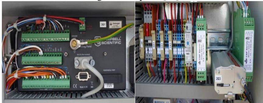
Fig. 8: Data logger. Figure 8: Connectors, GPRS modem, automatic switch [22]
